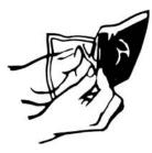
Thoroughly mix by squeezing Compound back and forth 30 to 40 times. Strip Compound from corners-while mixing.
