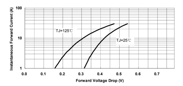
Fig.3-Typical Instantaneous Forward Voltage Characteristics
