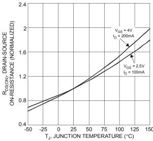
Figure 6 On-Resistance Variation with Temperature
